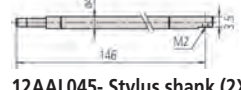
12AAL045 - Stylus shank (2X-long groove) For mounting CMM stylus (mounting thread M2)
