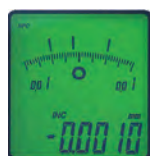
The display switches from green to red backlight if the upper or lower tolerance limit is exceeded
